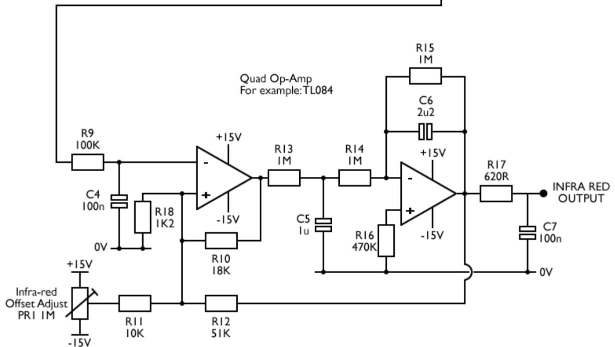
This circuit is based on the famous Polyfusion modular synthesizer Random Signal Generator, module 2002.
